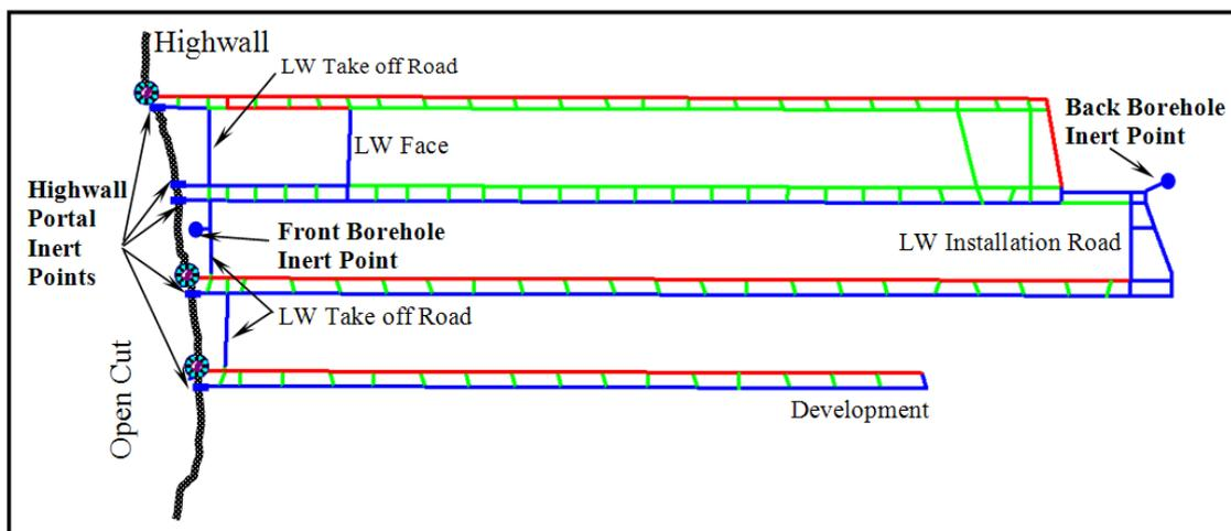
Figure 8 Typical punch mine layout and potential inert gas delivery points
