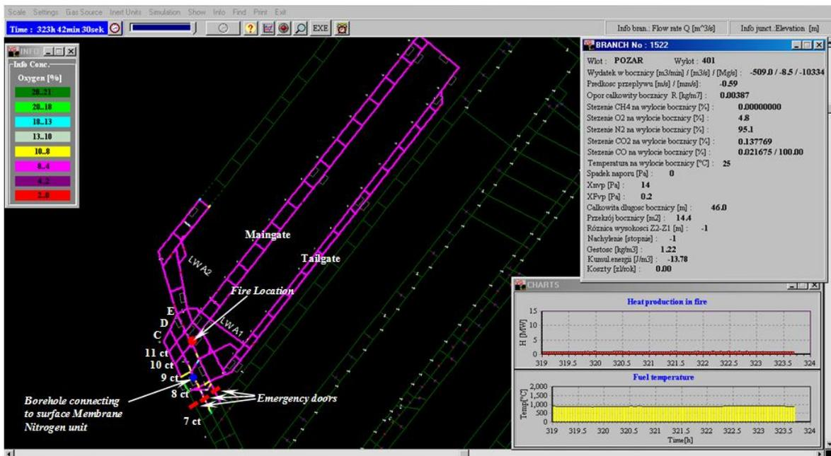
Figure 3 Oxygen distribution after 323 hours in the sealed area with combined control actions of closing emergency doors, short-circuiting and running the Membrane Nitrogen System.
